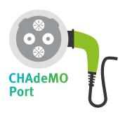
Some early EV models use a CHAdeMO port for DC Charging located next to the Type 2 port. The cable will be attached to the charger
