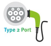
For AC charging, a Type 2 port and cable are used. This is the cable supplied with the EV.
