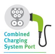
For DC charging a CCS port is used, built into Type 2 port. The cable required will be attached to the charger.
